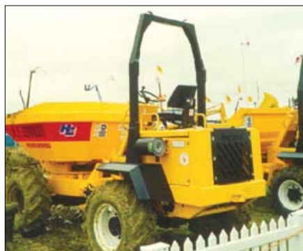
Figure 54 Site dumper with ROPS
