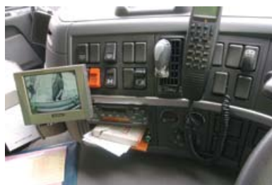
Figure 38 CCTV monitor in vehicle cab
